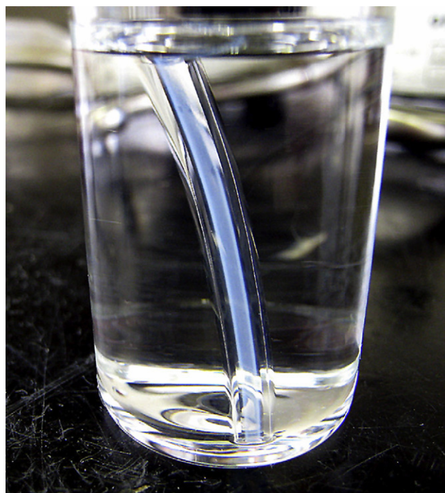
Fig. 10. Picture of PVC-g-PHEMA tube in THF. The inside of the tube appears white because the PHEMA that is grafted to the interior chains is not soluble in THF.
